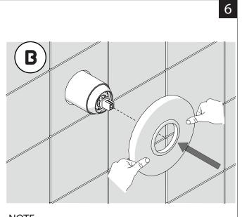
NOTE: Seal the faceplate to the wall using a suitable sealant
